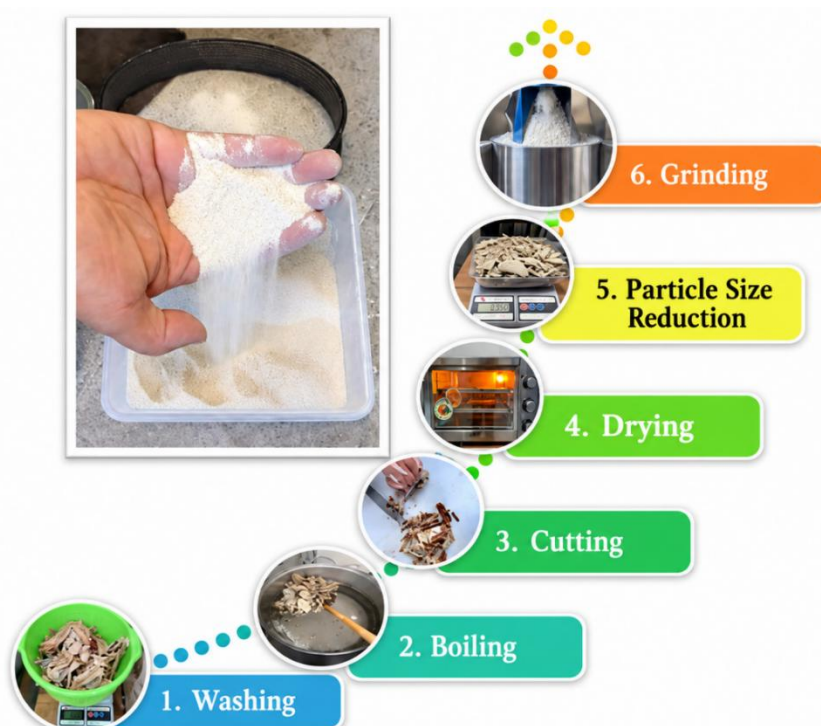
Figure 2. Process flow of raw material preparation showing sequential steps from washing, boiling, cutting, drying, particle reduction, to grinding. Each stage represents the transformation from coarse raw material into fine powder form used for further processing.
